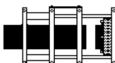
5. PIPE WITH SHORT SPIGOT STUB END
