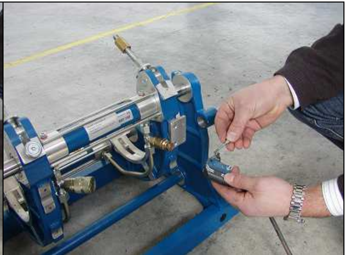
With the appropriate screws fix the microswitch
